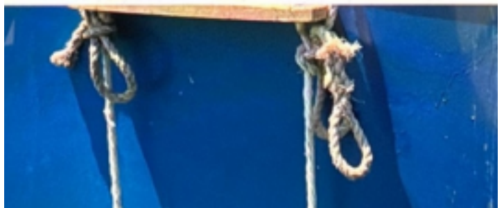
Non-compliant pilot ladder
