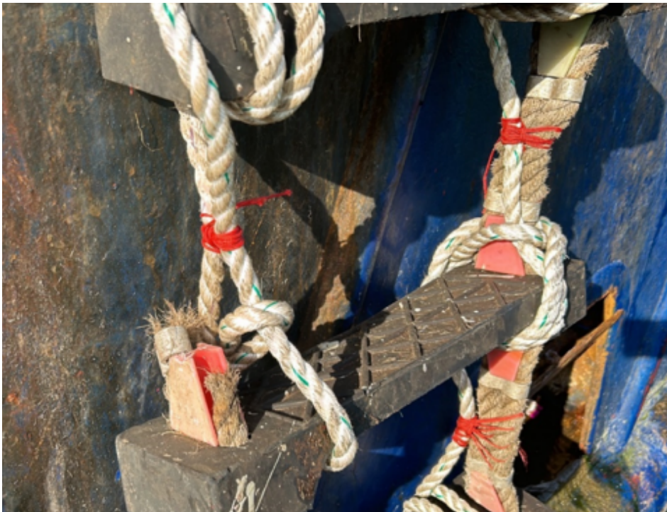
Defective Pilot Ladder
