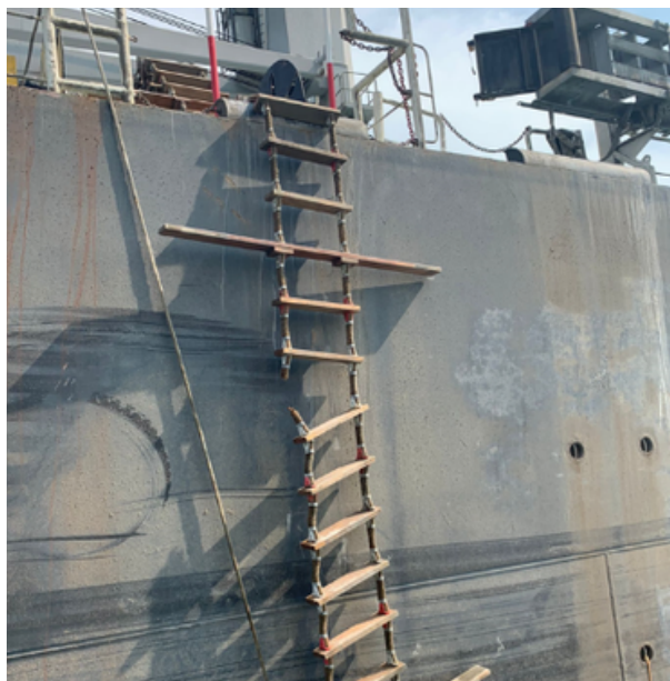
Damaged Pilot Ladder
