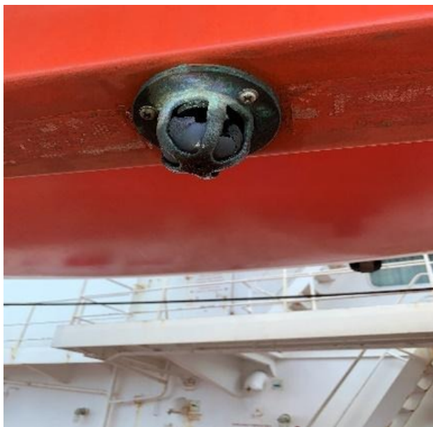
Broken Lifeboat Drain Plug
