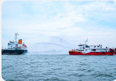
SCDF vessel sprayed "water curtains" to disperse plumes
