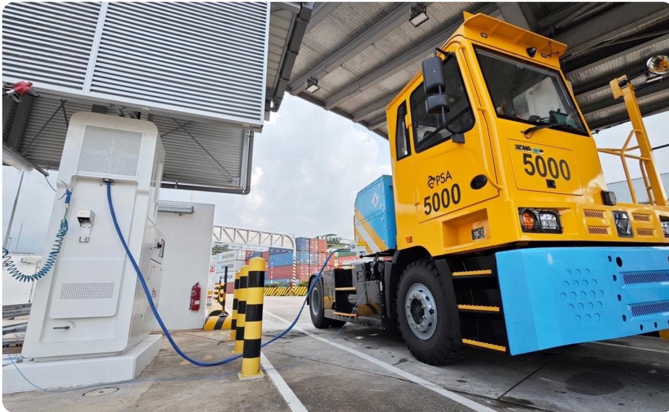
Hydrogen fuel cell electric prime mover at Pasir Panjang Terminal (Photo credit: PSA Singapore)
