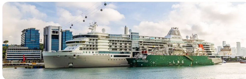
LNG bunkering at a passenger cruise terminal in Singapore on 24 February 2025 (photo credit: TotalEnergies)
