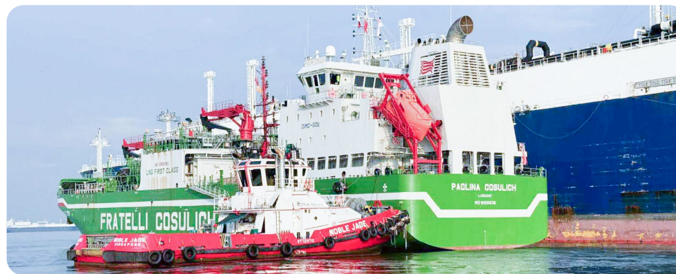
LNG bunker vessel positioned alongside an LNG carrier to receive fuel
