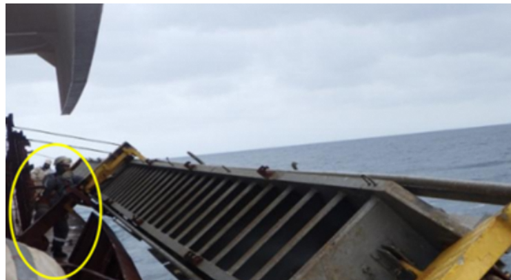
Fig. 11: The yellow circle highlights the BOS's position prior to the PAL being levelled with the deck.
