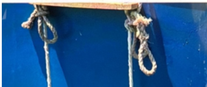
Non-compliant pilot ladder
