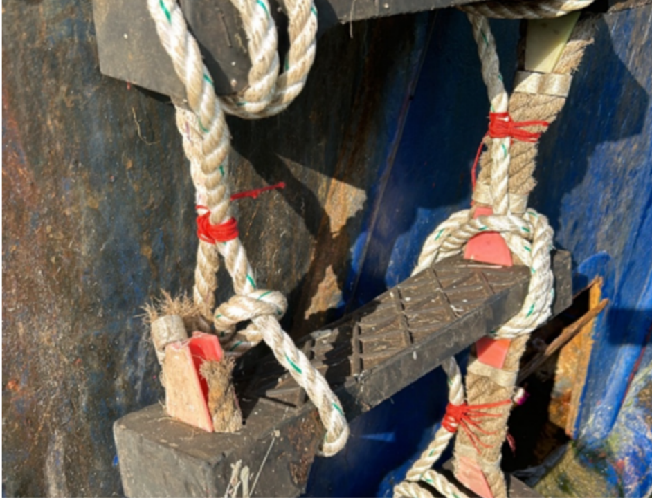
Defective Pilot Ladder
