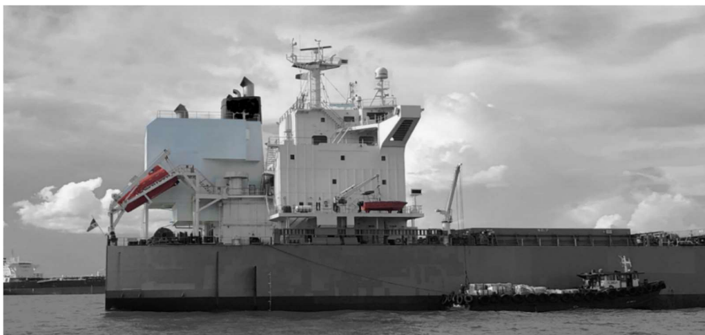
A bulk carrier retrofitted with enlarged funnel structure for scrubber
