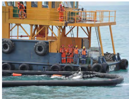
JOSE 2012: Recovery of oil using a heavy duty oil recovery system.
