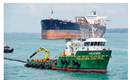
Dispersant-spraying craft combating the oil spill (top) and the deployment of a heavy-duty oil recovery system (above).
