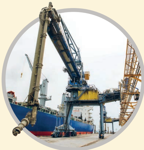
RIGHT: The air-slide conveyor system allows air to be pumped through the pipes along with cement.
