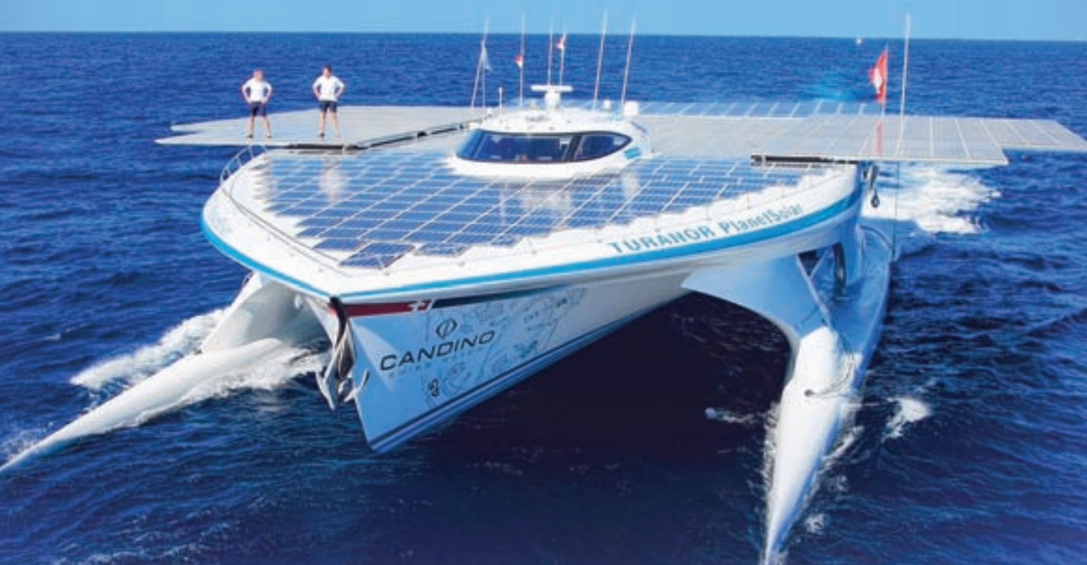
Stretching wings: Can be adjusted to get extra solar surface or reduce boat size when mooring.
