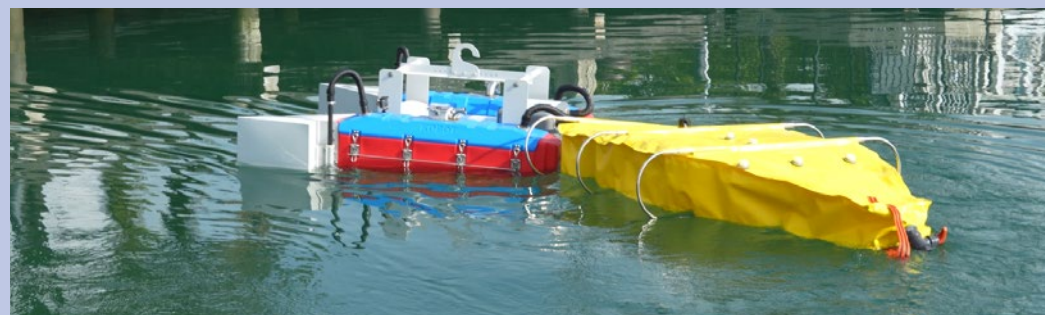
The KOBOT is designed for use in shallow, confined waters such as marinas and canals. It measures 4.5 by 1.5 meters and weighs about 160 kg.
