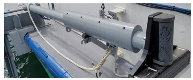
Joint innovation between MPA and contractor to design a streamline bracket on the sonar transducer pole that increases the streamline factor and reduces the vibration.
