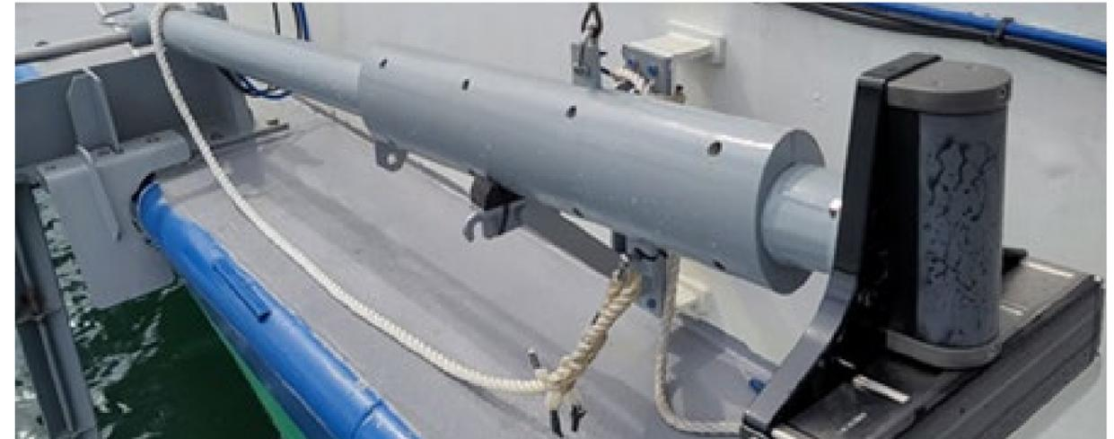
Joint innovation between MPA and contractor to design a streamline bracket on the sonar transducer pole that increases the streamline factor and reduces the vibration.
