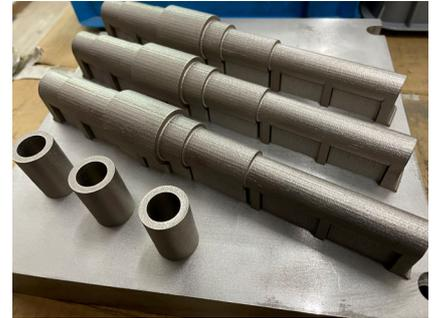
Figure 1: Printed Shaft
