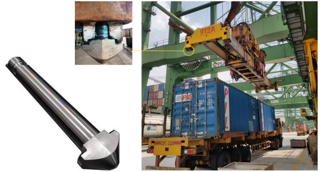
Figure 9: WAAM Twistlock Pin (left), and Operational use of WAAM Twistlock Pin (right)
