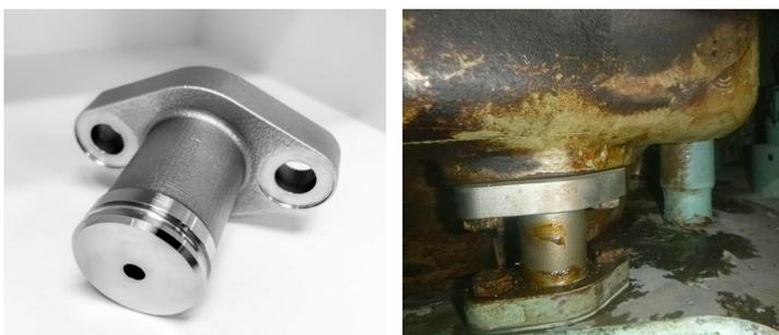
Figure 6: Printed cooling water pipe connector (left), and installation onboard bulk carrier (right)
