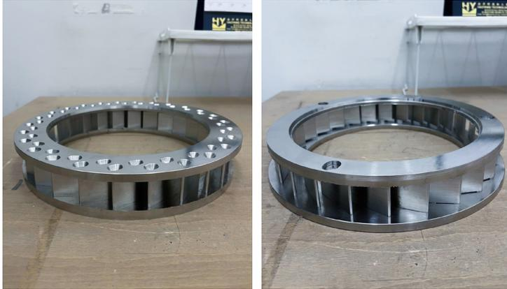
Figure 5: Top and bottom views of AM printed turbocharger nozzle ring
