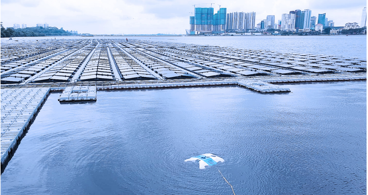
The A.IKANBILIS is an autonomous underwater vehicle designed to eliminate the risks and high costs of underwater inspections. Its sensors and AI features enable improved productivity and robust data collection in high-current and low-visibility conditions, while in-built batteries and an on-board processing unit support self-sufficient deployment.
