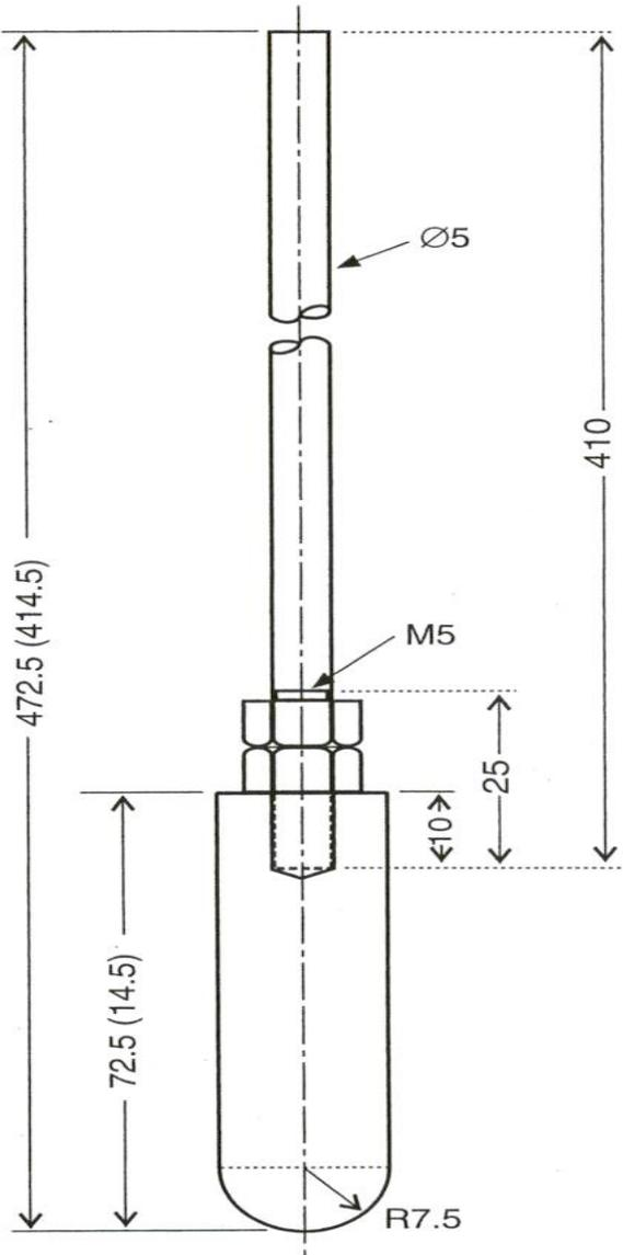
(Dimensions indicated in brackets are of the 5 kPa bit)
