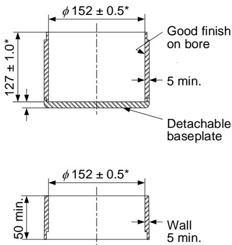
CBR Mould compaction cylinder and screw-on extension piece (from BS 1377 Part 4.
