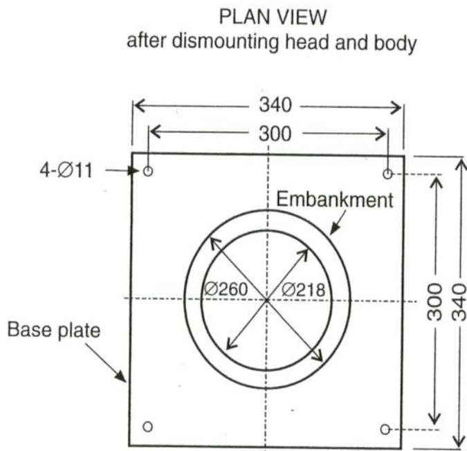
Figure 1.2.2.3-2 – Cylindrical vessel, 200 mm diameter
