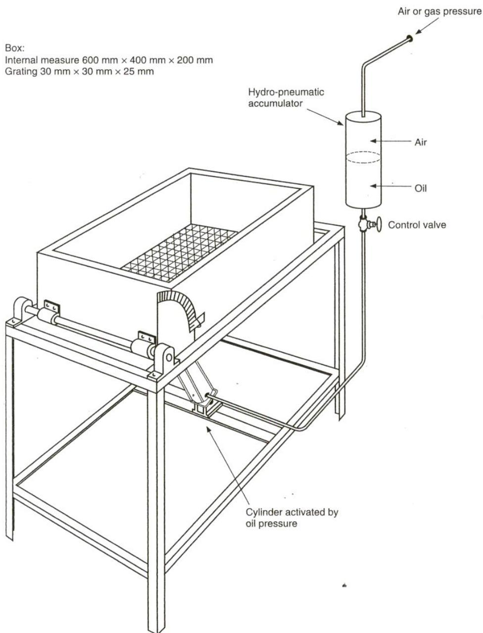
**Figure 2.1.4 – Basic sketch of tilting box**
