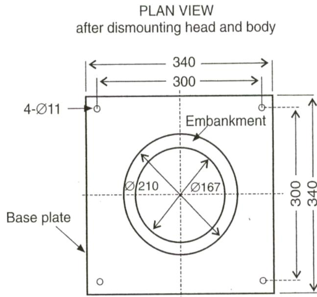
**Figure 1.2.2.3-1 – Cylindrical vessel, 150 mm diameter**
