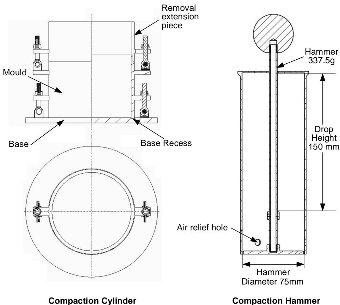
Figure 1.5.5.1.3.2 – Schematic of a Proctor/Fagerberg apparatus
