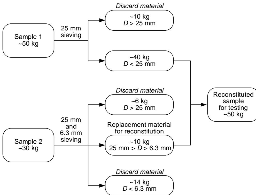
**Figure 1.6.4.3 – Schematic diagram of reconstitution sample procedure**
