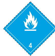
(No. 4.3) Class 4.3 Substances which, in contact with water, emit flammable gases Symbol (flame): black or white. Background: blue. Figure '4' in bottom corner.
